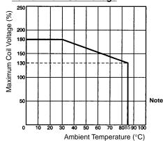
The maximum coil voltage refers to the maximum value in a varying range of operating power voltage, not a continuous voltage.
