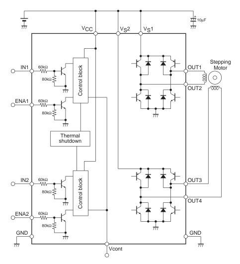
Note: As long as the voltages applied to V<sub>CC</sub>, V<sub>S</sub>1, V<sub>S</sub>2, ENA1, ENA2, IN1, and IN2 are within the limits set by the absolute maximum ratings, there are no restrictions on the relationship of each voltage level in comparison with the others (regarding which is higher or lower). (ex. V<sub>CC</sub> = 3V, V<sub>S</sub>1, 2 = 2V, ENA = IN = 5V)
