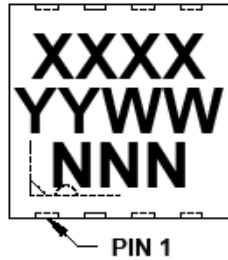
8-Lead DFN (3x3 mm)
