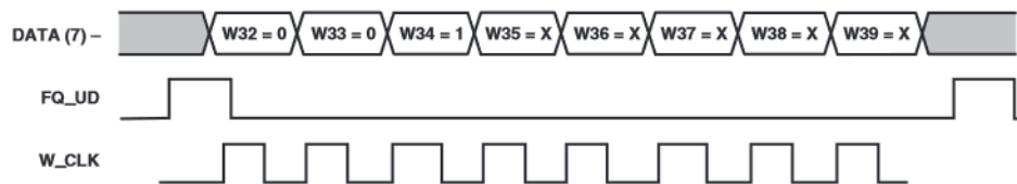
Figure 13. Serial Load Power-Down Sequence
